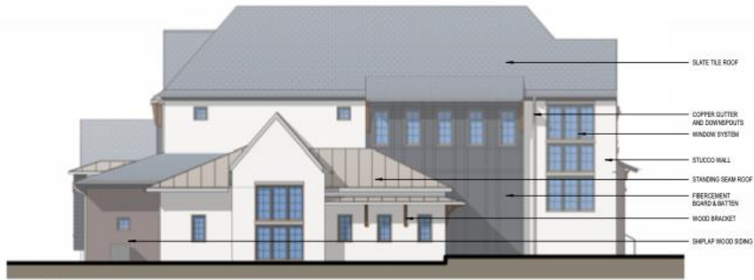
2 ESTATE HOME - SIDE ELEVATION (GARAGE) P301 SCALE: 1/8" = 1'-0"
