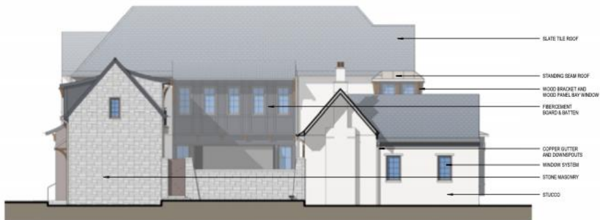
3 ESTATE HOME - SIDE ELEVATION (TERRACE) P301 SCALE: 1/8" = 1'-0"
