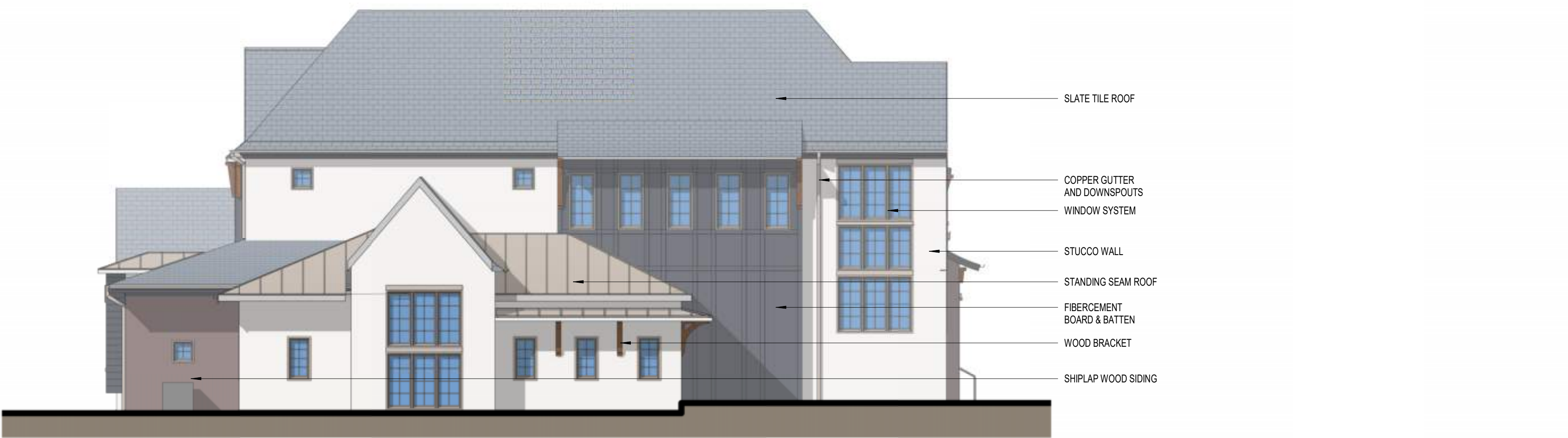
2 ESTATE HOME - SIDE ELEVATION (GARAGE) P301 SCALE: 1/8" = 1'-0"
