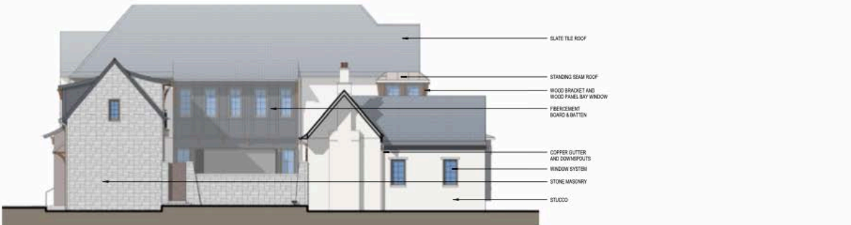
ESTATE HOME - SIDE ELEVATION (TERRACE)
