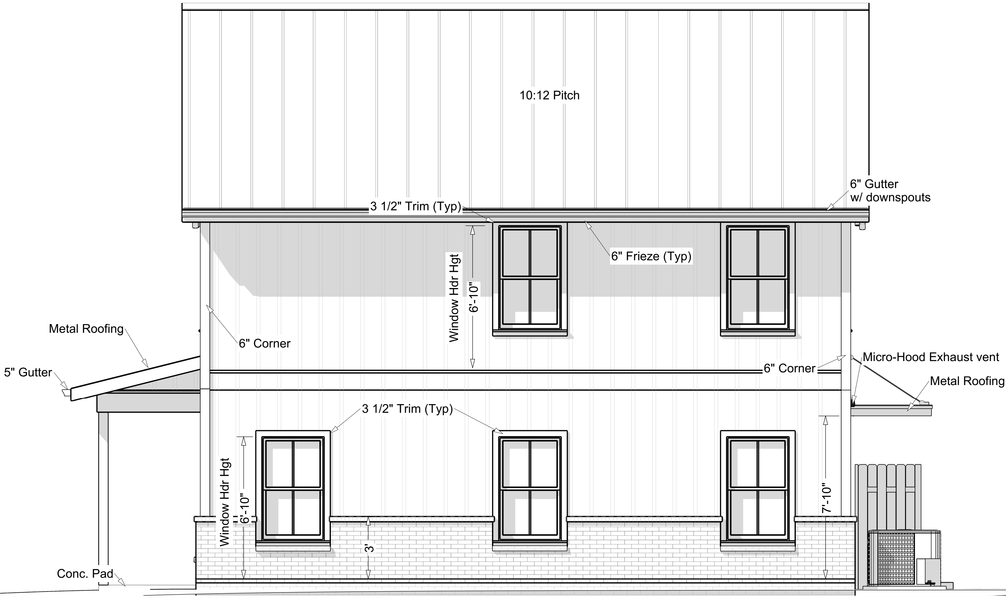
Exterior Elevation Right
