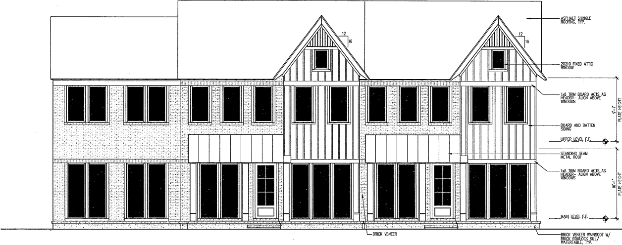
1 FRONT ELEVATION— BUILDING 4 A303 1/4"=1'-0"
