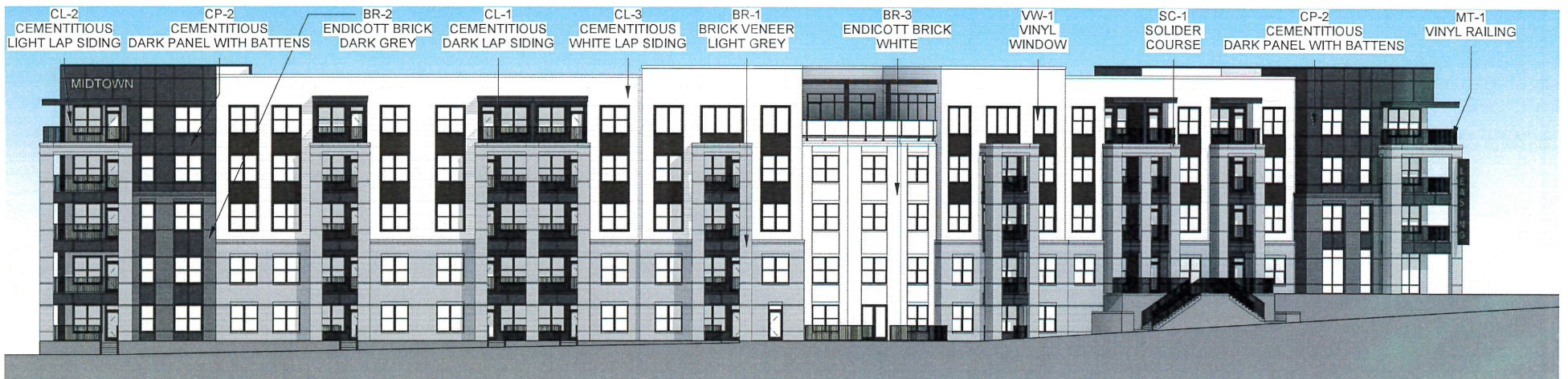
BLDG 2000 - FRONT ELEVATION
