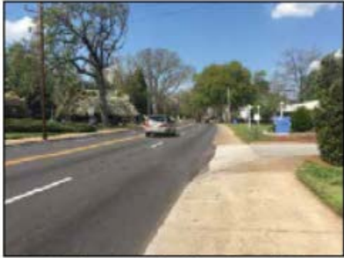
No separation between the sidewalks and the street; in some places, the sidewalk is the same level as pavement
