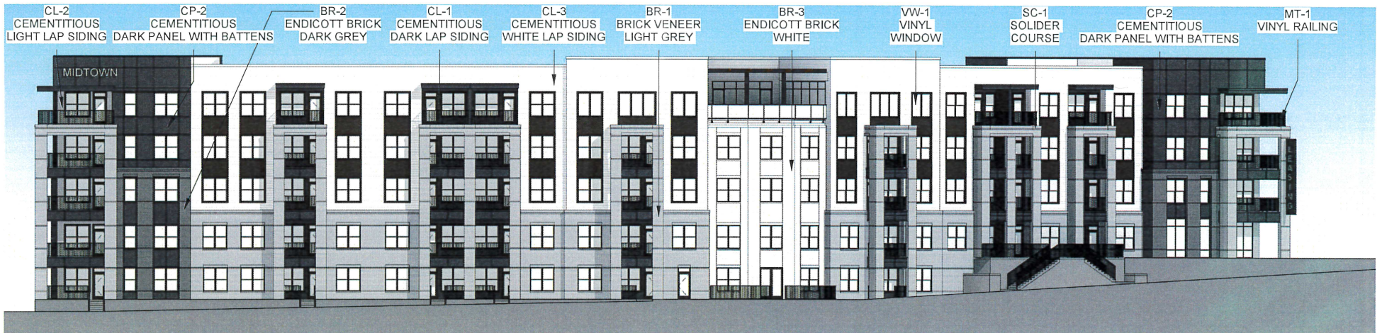
BLDG 2000 - FRONT ELEVATION
