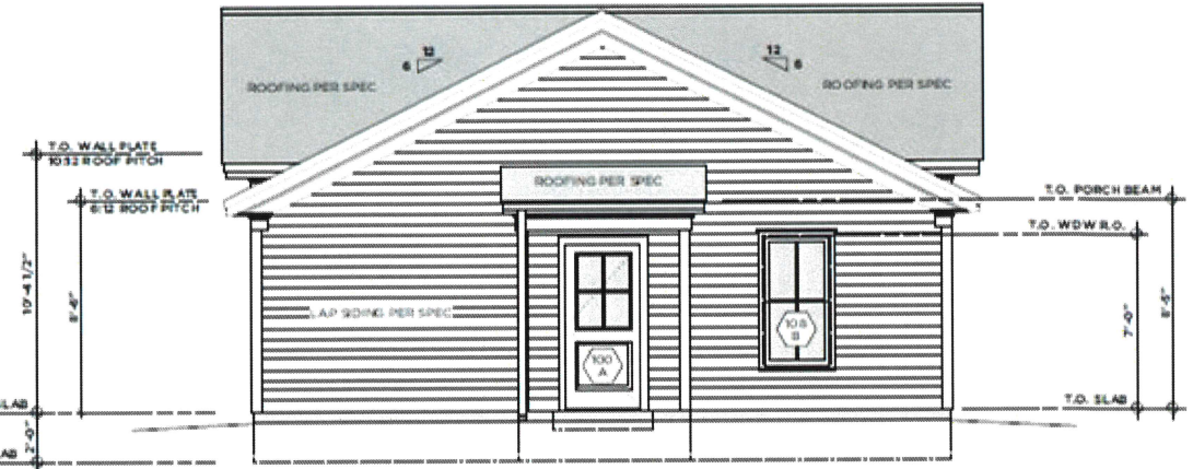
REAR ELEVATION ③ SCALE 1/4" = 1'-0"
